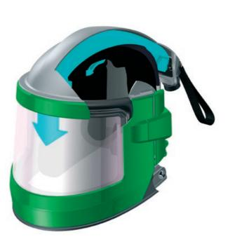
distribution of airflow brings air to the breathe zone and reduces lens fogging. The air channel stops head chill and directs the air where it's needed! Vents in the top dome allow air to also pass around the head for extra comfort. This engineering is supported by a fail-proof air tube attachment that can only be assembled the correct way, limiting time for re-adjustments and removing the risk of malfunction.
